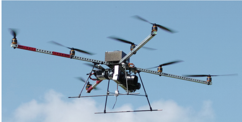
Figure 1: UAV Multirotor MR-X8 with Sigma DP2 sensor head.
