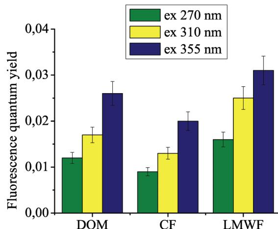
*Figure 9: The fluorescence quantum yield of DOM, its colloidal fraction (CF) and its low molecular weight fraction (LMWF).*
