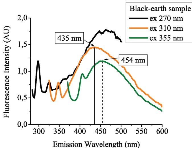
Figure 3: Emission spectra of soil aqueous extractions under excitation at 270, 310 and 355 nm.
