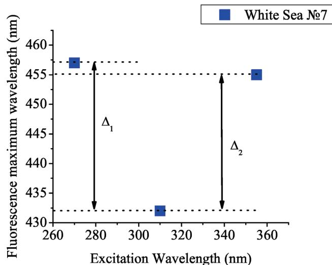
*Figure 2: Fluorescence maximum wavelength dependence on excitation of marine water samples with schematic view of  $\Delta_1$  and  $\Delta_2$  values.*
