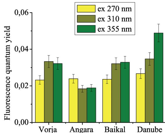
Figure 6: The fluorescence quantum yield dependence on excitation of fresh water samples.
