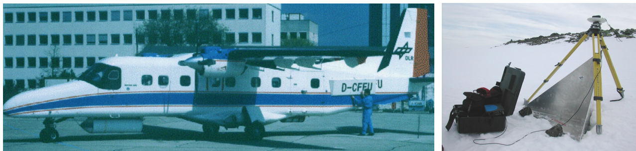
Figure 2, Left: ESAR aircraft. Right: Corner reflectors and GPS equipment for accurate differential GPS measurements.
