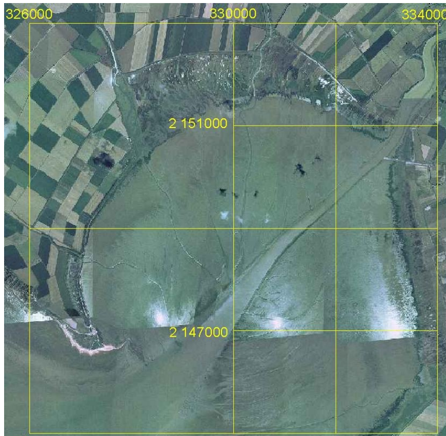
Figure 4: Orthophotograph of Aiguillon cove (August 2, 2000) and extensions of photogrammetric DTM calculations. Coordinates are in the metric Lambert system.
